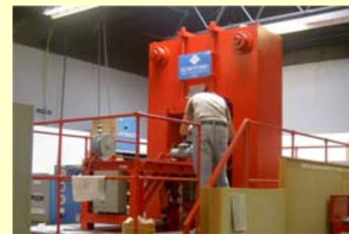
Fig. 2 SPS (GM, not shown) and Hot Press Max. rate 300°C/s, Max. P = 4000 Kbar, Max. T = 2500°C at BNL and SBU
