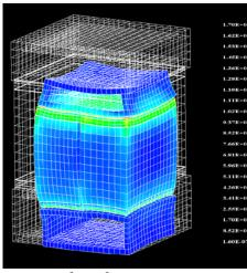
Stresses back at room temperature after fabrication
