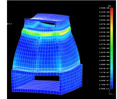
Stresses when operating across large  $\Delta T$ Bonded to hot and cold side heat exchangers
