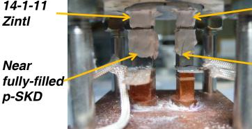
High Temperature Segmented Zintl/La<sub>3-x</sub>Te<sub>4</sub>/SKD Couple Spring-loaded Performance Test Configuration
