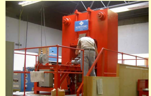
Fig. 2 Hot Press Max. rate 300°C/s, Max. P = 4000 Kbar, Max. T = 2500°C at BNL and SBU
