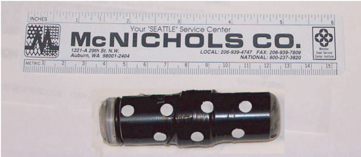
Figure 4.2. A three degree-of-freedom Sensor Fish wrapped with black tape and marked with white stickers.
