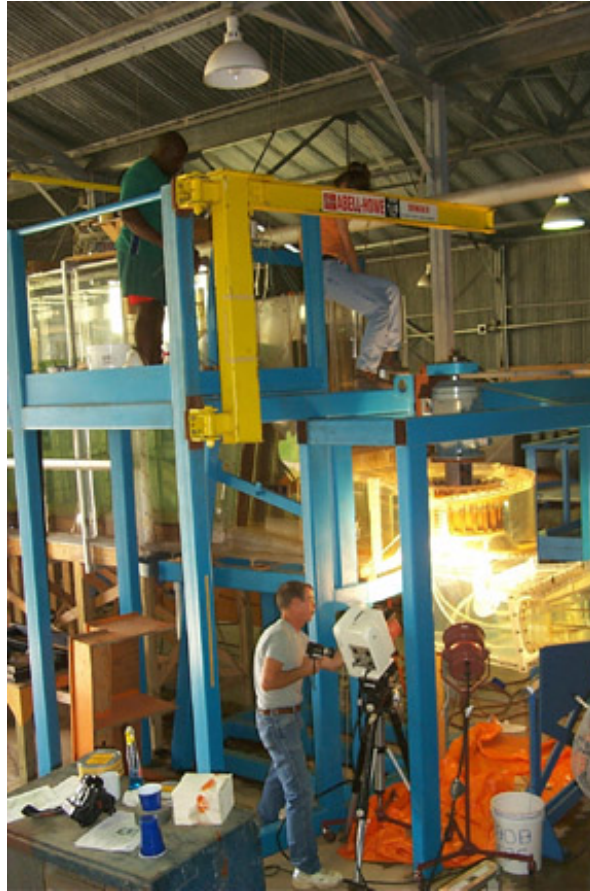
Figure 15-Setup of high-speed film cameras and Model at ERDC.
