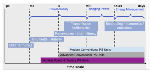
Figure 3-6 Timeframes for advanced pumped storage unit regulation
