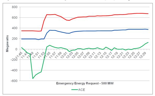
Figure 3-5 Pumped storage units balancing forecast error
