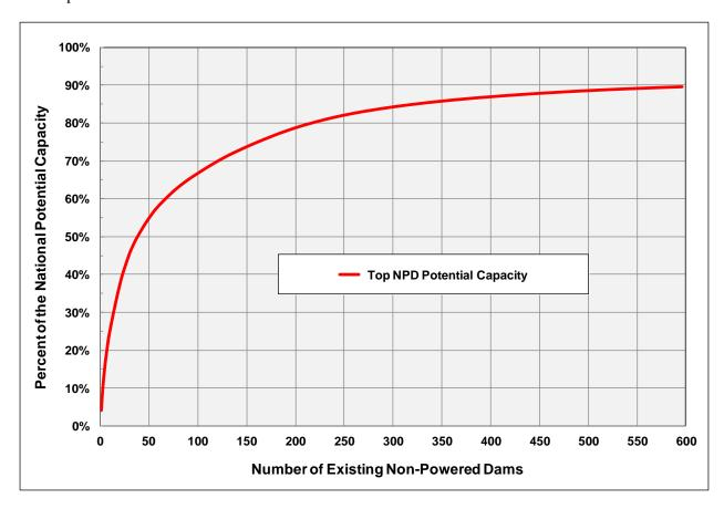
Figure 10. Cumulative potential capacity distribution of the top existing NPDs with the greatest potential added generation capacity
