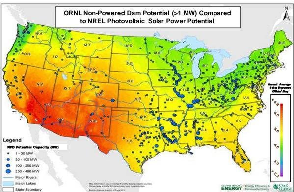
Figure 13. Comparison of top NPD sites with potential capacities greater than 1MW with maps of wind and solar photovoltaic resource potential
