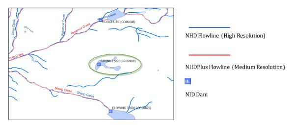
**Figure 4. Illustration of the second criterion for selecting DWNS** – In this example, because the dam "Crane Lake" is not close to any NHD flowline or NHDPlus flowline, it cannot be linked to any stream and is designated as located on segment with negligible streamflow.
