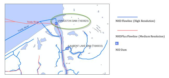
**Figure 5. Illustration of linkage between NID and NHDPlus** – In NID, Livingston Dam is linked to an NHDPlus flowline (in red color), which represents the Trinity River. The accumulative drainage area for this NHDPlus flowline is 16,572 square miles, which will be used as the dam's drainage area.
