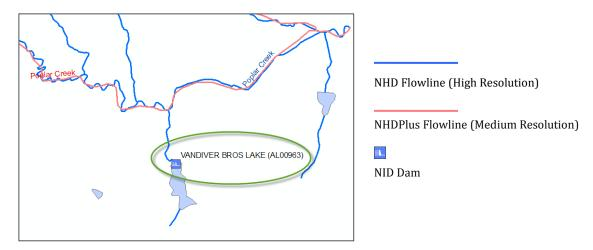
**Figure 3. Illustration of the first criterion classification of DWNS** – In this example, because the dam "Vandiver Bros Lake" is close to NHD flowline but far from NHDPlus flowline, it is designated as located on segment with negligible streamflow.
