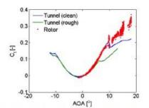
Normal force (left) and tangential force (right) coefficient vs. AOA. Blue curve is tunnel measurements on a clean airfoil, green curve is tunnel measurements on an airfoil with leading edge roughness and red dots are measurements at r=20m on the rotor.
