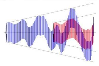
The wakes from two turbines (or more) only rarely coincide. Even in full wake direction, the path's will be different.
