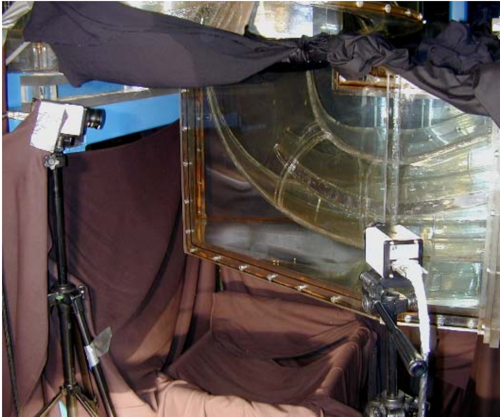
Figure 2.7. Camera positioning in relation to the elbow and splitter region of the model.
