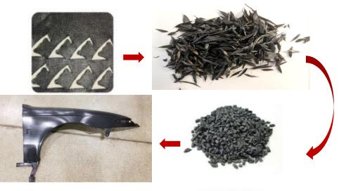
CARBON FIBER FILLED THERMOPLASTIC
