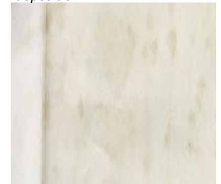
graphite + 10% COphite Material w/ minimal Li deposition
