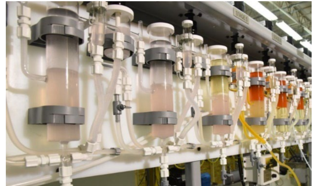
Solvent Extraction Testbed Facility with centrifugal contactor system
