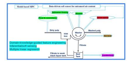
Purdue and industrial partners created an **ABET accredited 4-yr BS Degree program** focused on SM technologies integrated with state-of-the-art facilities with industry grade equipment ML Based Soft Sensor for Entrained Air Content in Browstock Washing (Pulp and Paper) reduced defoamer usage by 35% and water usage by 10%
