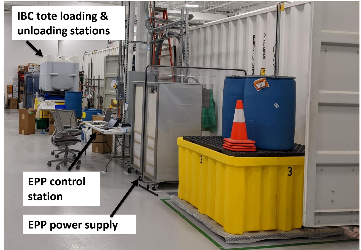
A picture of LCE's electrolyte-purification process (EPP) system housed inside a 53-foot shipping container in LCE's facility in Wilmington, MA
