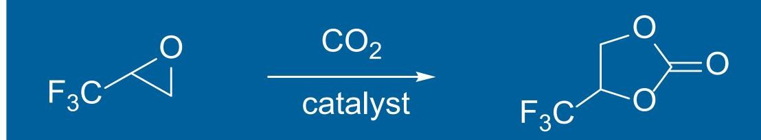
Argonne developed "green", atom efficient synthesis of TFPC in continuous flow reactor
