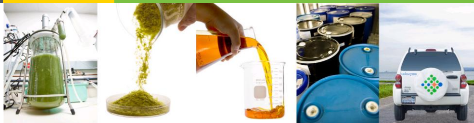
Left to right: (a) Laboratory scale fermentation of algae (b) Dried algal biomass (c) Purified algal oil (d) Thousands of gallons of algal oil have been produced in nonintegrated tolling facilities. Solazyme algal oils have been refined to transportation fuels that meet industry specifications. (e) Solazyme’s biodiesel and renewable diesel have powered a light truck and three cars with unmodified diesel engines for thousands of miles on the open road (with blends ranging from B20 to B100).
