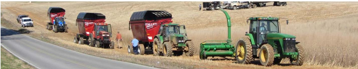
A pull-type forage harvester, tip wagons, and trucks stand ready for harvest at the edge of a switchgrass field. The harvester (scalable for commercial use) creates the bulk format, and the tip wagons and trucks collect the loose bulk format for transport to nearby storage. Bulk compaction increases the density of low-moisture switchgrass for transport over longer distances. *Photo: Al Womac*
