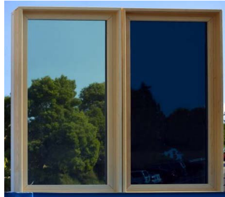
Prototype – Concept Window Highly Insulating and Dynamic SHGC 0.04 – 0.34
