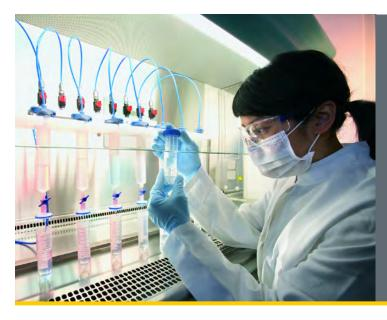
With no new equipment to install or repair, proper fume hood management along with user training is an effective energy savings measure with a quick payback. Decommissioning and consolidating fume hoods can greatly decrease the amount of wasted energy due to open fume hood sashes.
