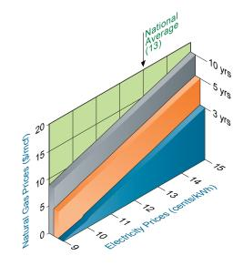
Shown here are natural gas and electricity prices needed to achieve three-, five-, and 10-year simple paybacks for a 2 MW CHP system. At an electricity price of 13 cents/ kWh, a five-year simple payback can be achieved when natural gas prices are less than \$11.25/mcf.
