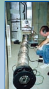
Duct leakage is tested using a duct blaster.
