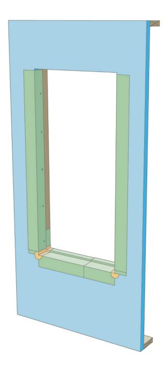
Apply sealant at jambs and head; alternatively, sealant can be placed on the backside of the nailing flange (backcaulked); sealants, housewraps, and flashings must be chemically compatible
