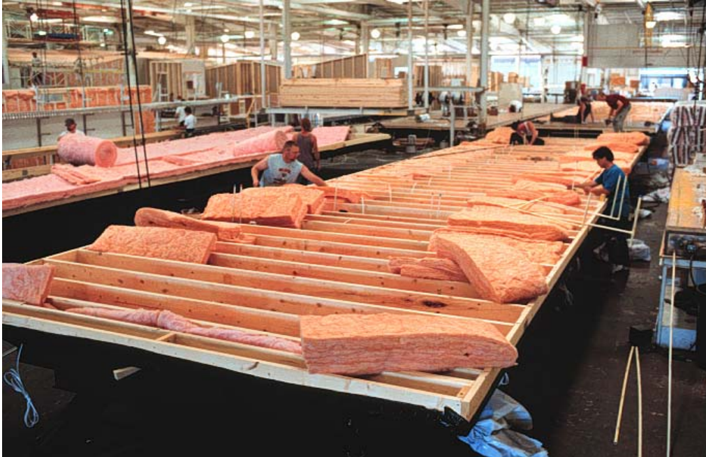
Figure 39. NEEM home floor assembly, Fleetwood Homes of Washington
