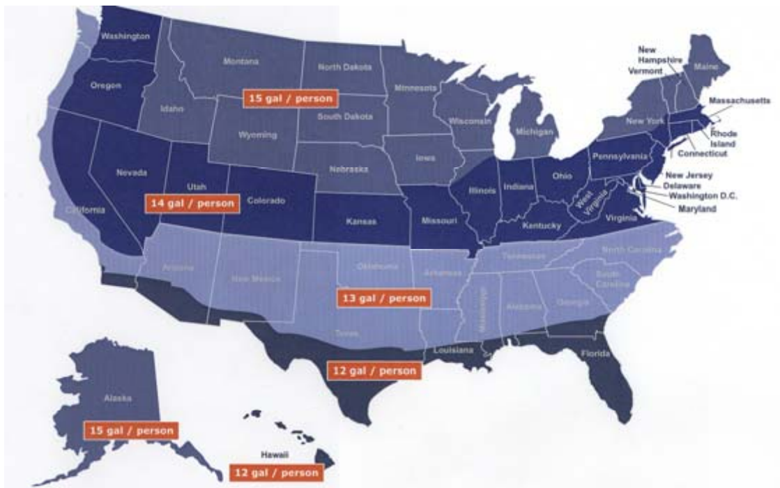
Figure 18. Domestic hot water tank sizing for 135°F tank temperature only
