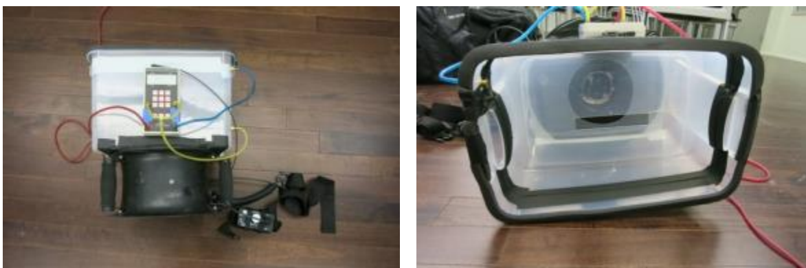
Figure 9. Testing device for passive vents
