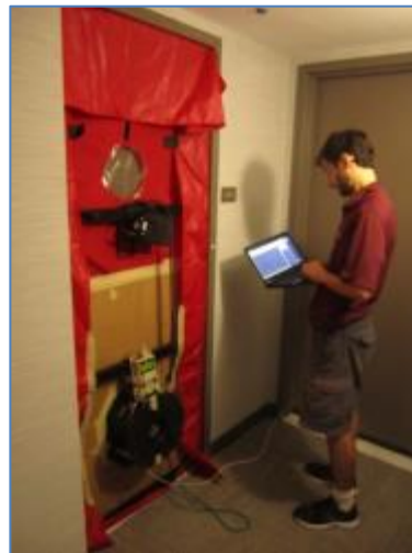
Figure 1. Measuring leakage area of entry door
