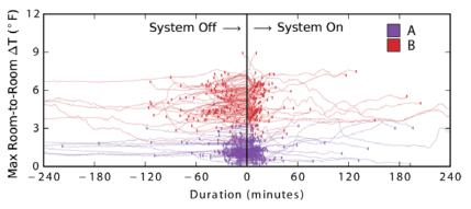
Plotting can aid in the analysis of systems. Differences in indoor conditions between the two homes become clear when all of the HVAC systems' cycles are displayed in unison and are color coded.
