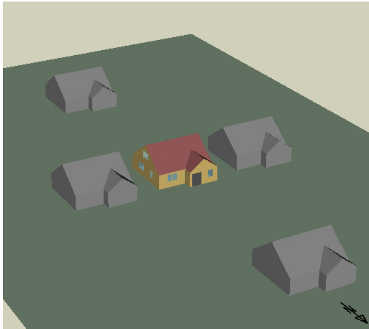
Figure 22. BEopt model orientation, geometry, and neighboring structures
