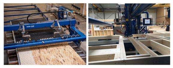
Figure 5. Timber frame manufactured with robotic exterior cladding application (left) and CNC machine (right)
