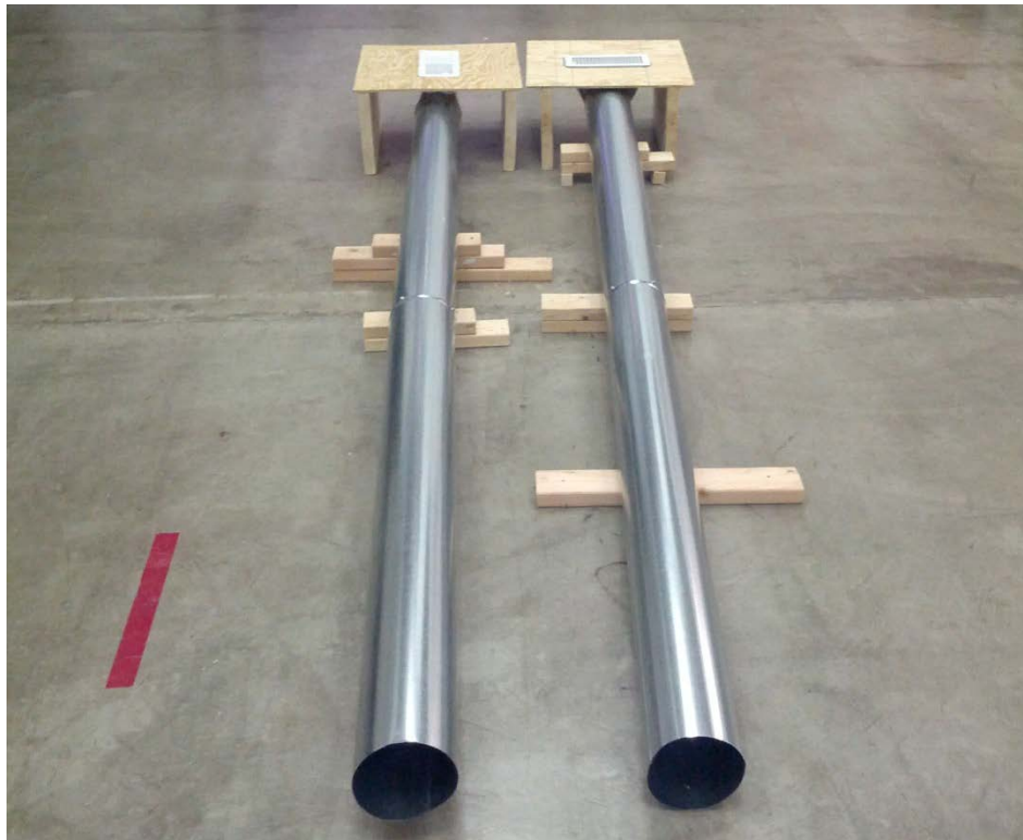
Figure 2. Mockup of the testing duct runs
