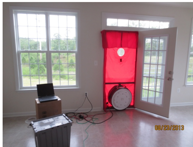
Figure 4. Location of the house-to-outdoors fan pressurization testing equipment
