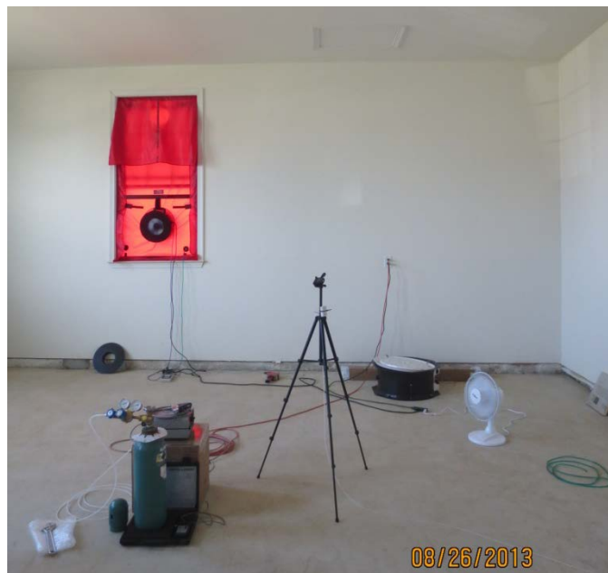
Figure 9. Testing equipment located in the garage: SF 6 tracer gas on a scale and mass flow controller for tracer gas injection (lower left); calibrated fan for garage exhaust (upper left); garage air concentration and temperature/RH sampling station (tripod in center); mixing fan (right); garage air pressure sampling tube (far right)
