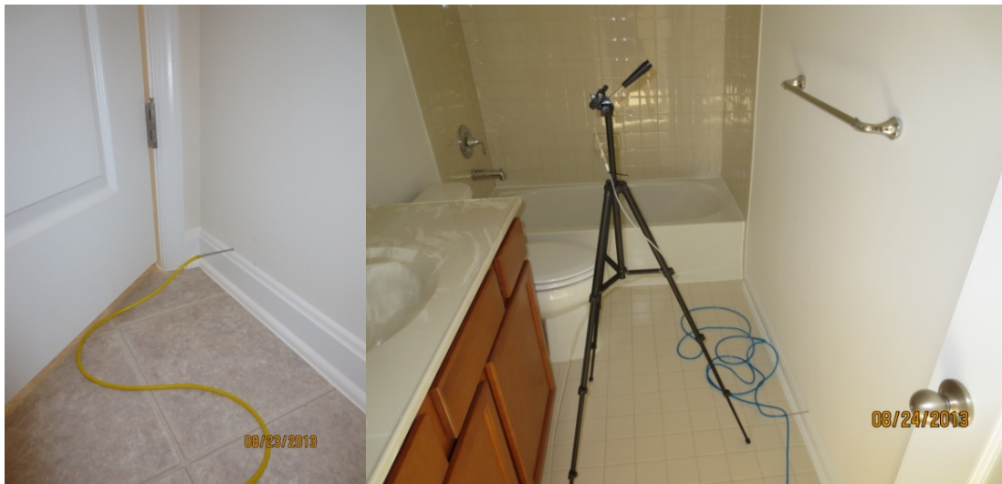
Figure 7. First-floor garage-to-house wall cavity pressure measurement location, and second-floor garage attic-to-house wall cavity pressure measurement and room air sampling location
