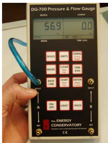
Figure 17. Pressure mapping can be performed using a manometer.
