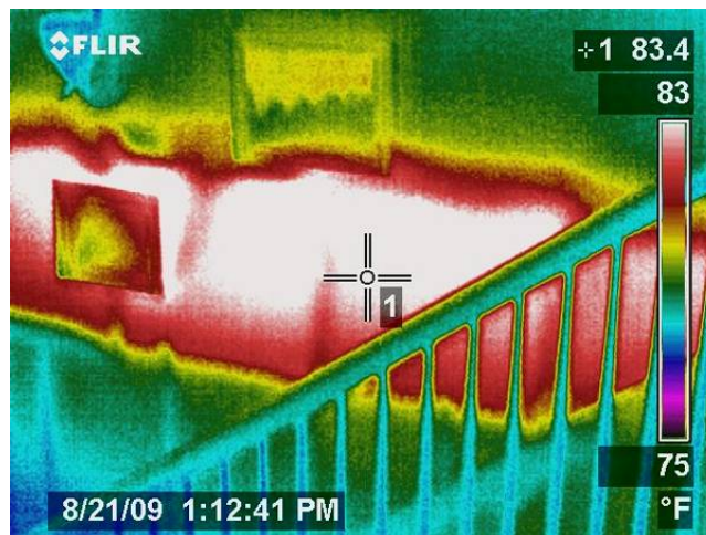
Figure 13. Infrared image of stairwell showing elevated wall temperature from hot air in an interstitial floor cavity. Note location of pictures and light fixture.
