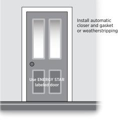
Figure 18.1. Use backer rod, caulk, or nonexpanding foam approved for windows and doors to fill the rough-in gap around doors and windows (DOE 2000). Figure 18.2. Install automatic closer and gasket or weather stripping around doors. Caulk around trim.
