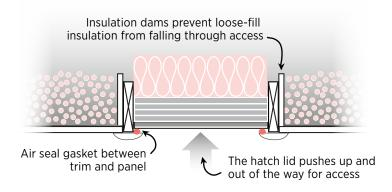
Figure 9.2. Insulate and air seal the pull-down attic stair.
