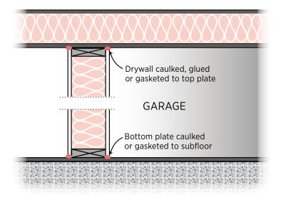
Figure 15.1. Finish the walls that separate the garage from the rest of the home with drywall that is sealed to the top and bottom plate with a bead of caulk.
