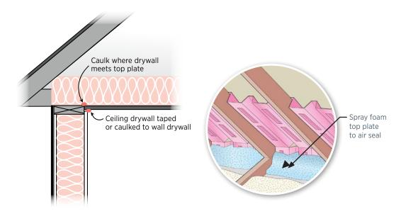
Figure 2.1. Seal the wall drywall to the top plate and ceiling drywall.
