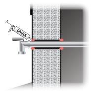
Figure 13.1. Caulk all plumbing penetrations through exterior walls.
