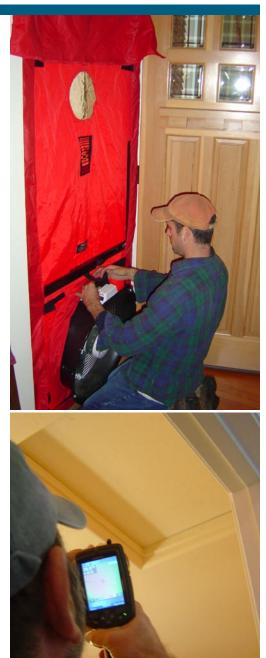
*(top)* Your contractor can use a blower door to measure overall house air leakage.
