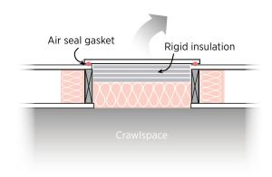
Figure 17.3. Air seal the crawlspace access hatch by installing a gasket or weather stripping around the hatch edges.
