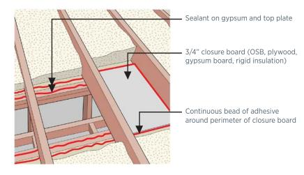
Figure 5.1. Place a solid air barrier over soffits as follows: pull back existing insulation; cover area with air barrier material (gypsum, plywood, OSB, rigid foam, etc.); seal edges with caulk; cover with insulation (Lstiburek 2010).
