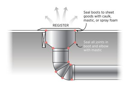
Figure 11.2. Mastic seal all supply and return air ducts.
