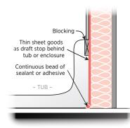
Figure 13.2. If you are remodeling a bathroom make sure you seal and insulate behind the tub or shower, especially if it is on an exterior wall.
