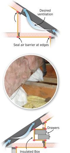
Figure 3.1. Insulate and air seal the kneewall itself, as shown, or along the roof line (Source: DOE 2000a).
