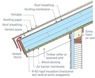
Building Science Corporation prepared this detail showing a home with rigid foam wall sheathing and a vented roof over a heavily insulated sealed attic.
