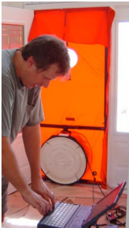
Figure 9.1. A Building America team member conducting a blower door air leakage test of a new home in Gainesville, Florida
