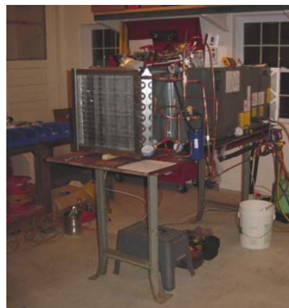
Bench-top testing of an advanced air conditioner with dehumidification mode (ACDM) in 2005
