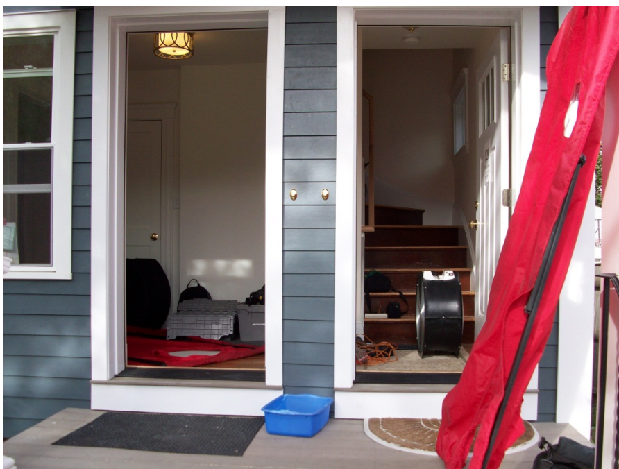
Figure 14. Belmont Two-Family: Setting up blower door testing
