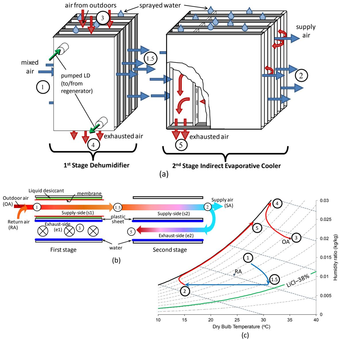
Figure 1: (a) Schematic of DEVAP a/c, (b) top view of channel pair, and (c) air states on a psychrometric chart. LiCl-38% is humidity ratio in equilibrium with 38% concentration LiCl.
