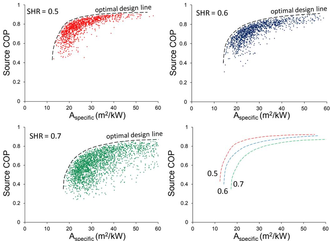
Figure 2: Source  $COP$  and specific area of each parametric analysis run. The bottom right plot shows the optimal design line for each  $SHR$ .
