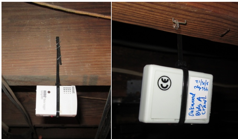
Figure 28. Example of the temperature and RH data logger left in each crawlspace to record data for the next year
