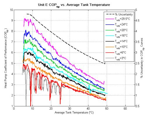
Figure 34. COP<sub>hp</sub> traces for Unit E
