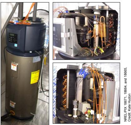
Figure 14. Unit B in the test plenum (left) and the instrumented heat pump components (right)
