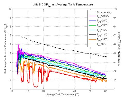
Figure 16. COP<sub>hp</sub> traces for Unit B
