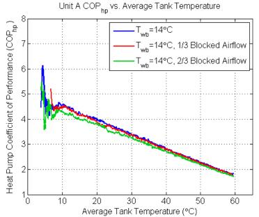
Figure 13. Heat pump COP<sub>hp</sub> traces for Unit A HPWH with reduced airflow
