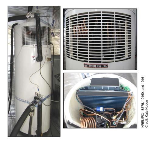
Figure 26. Unit D, an 80 gallon HPWH, installed in the test plenum (left). A close up of the air intake (top right) and the heat pump (bottom right) are also shown.
