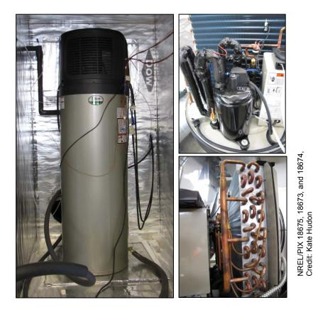
Figure 8. Unit A 80 gallon HPWH installed in test plenum (left). A close-up of the compressor and refrigerant system in Unit A (upper right) and a side view of the evaporator coils and heat exchanger (lower right).
