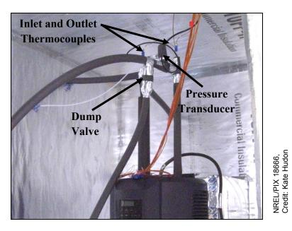
Figure 4. Inlet pressure transducer and thermocouple, outlet thermocouple, and dump solenoid valve on Unit B
