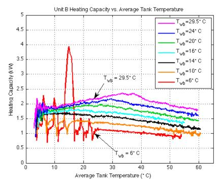
Figure 45. Heating capacity as a function of average tank temperature for Unit B
