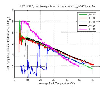
Figure 38. COP<sub>hp</sub> comparison for five HPWHs at 14°C inlet wet bulb air temperature
