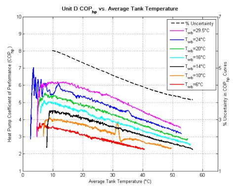
Figure 28. COP<sub>hp</sub> traces for Unit D
