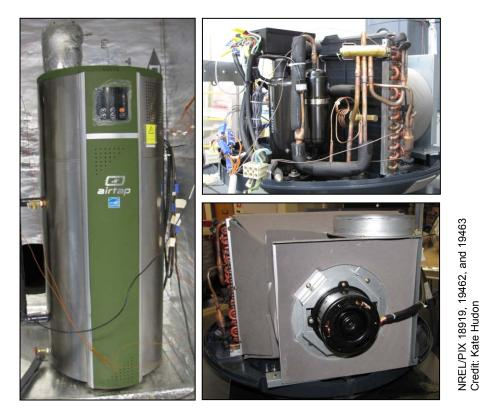
Figure 32. Unit E installed in test plenum (left). Some of the refrigerant system is shown (upper right), along with the blower that is designed to connect to a 6 in. duct (lower right)
