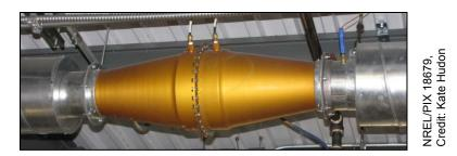
Figure 3. Laminar flow element used to measure airflow rates out of HPWHs
