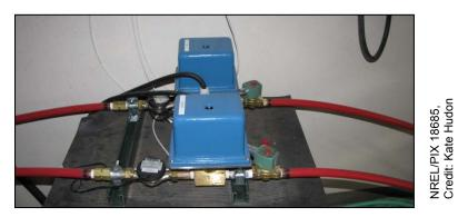
Figure 7. Outlet turbine flow meters, proportioning valves, and solenoid valves used to control outlet flow rate and draws
