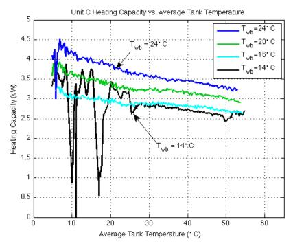
Figure 46. Heating capacity as a function of average tank temperature for Unit C
