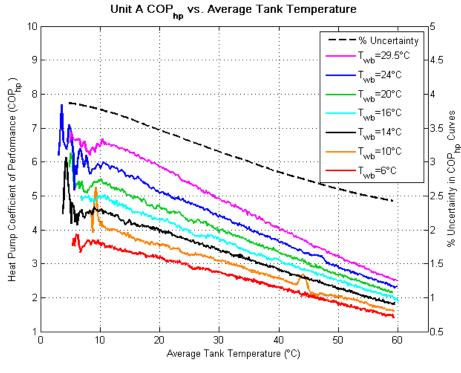
Figure 10. COP<sub>hp</sub> traces for Unit A
