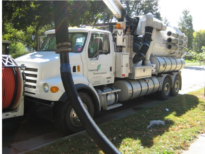
Figure 5. The hydrovac truck
