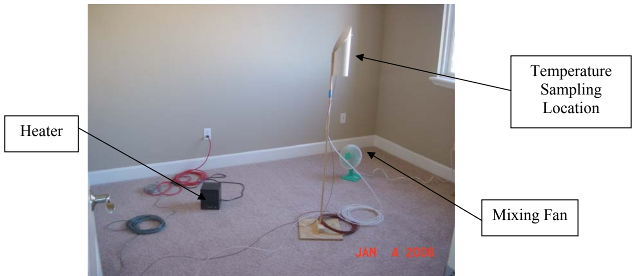
Figure 6. Tracer gas sampling point, temperature sensor, room air mixing and co-heating set-up.
