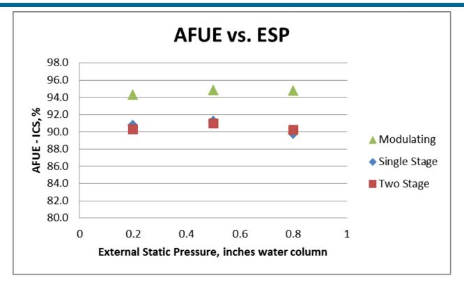
Figure 18. AFUE with varying external static pressure
