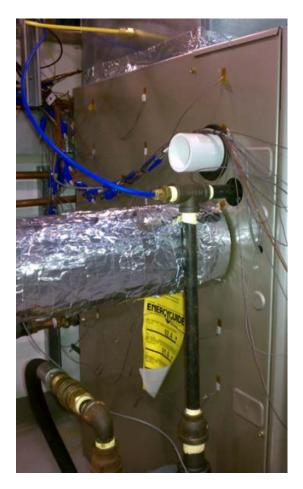
Figure 16. Furnace AFUE test showing jacket loss detail
