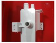
Figure 11. Condensate traps are gravity fed, the inlets must always be on the top
