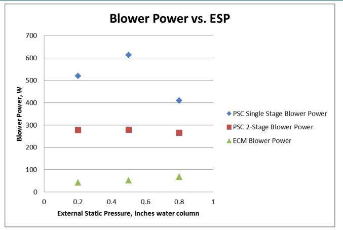
Figure 19: Blower power with varying external static pressure
