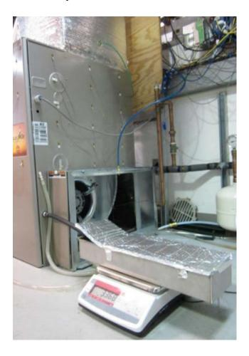
Figure 15. PARR AFUE lab testing
