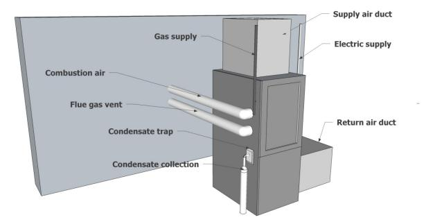
Figure 7. High efficiency furnace components
