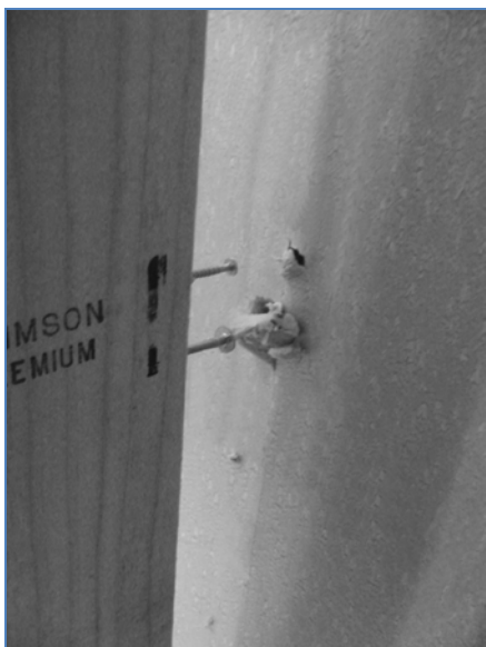
Figure 17. Group 4A failure mode, nail pull-through
