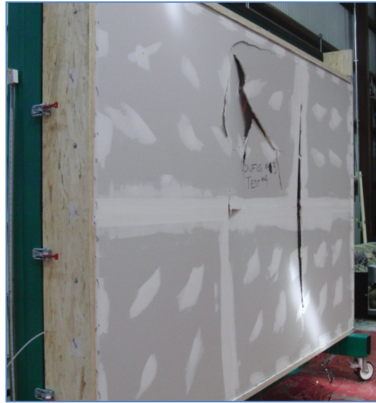
Figure 15. Group 3C failure mode
