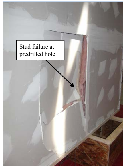
Figure 16. Group 3D failure mode
