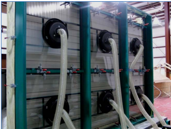
Figure 2. Testing frame with installed wall specimen
