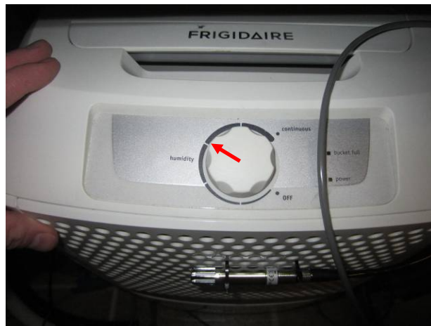
BDC houses: Dial on dehumidifier set to around 60% of lowest humidity setting, or 10 o'clock (red arrow indicates approximate setting)
