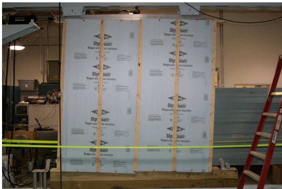
Figure 24. XPS sheets twisted in-plane
