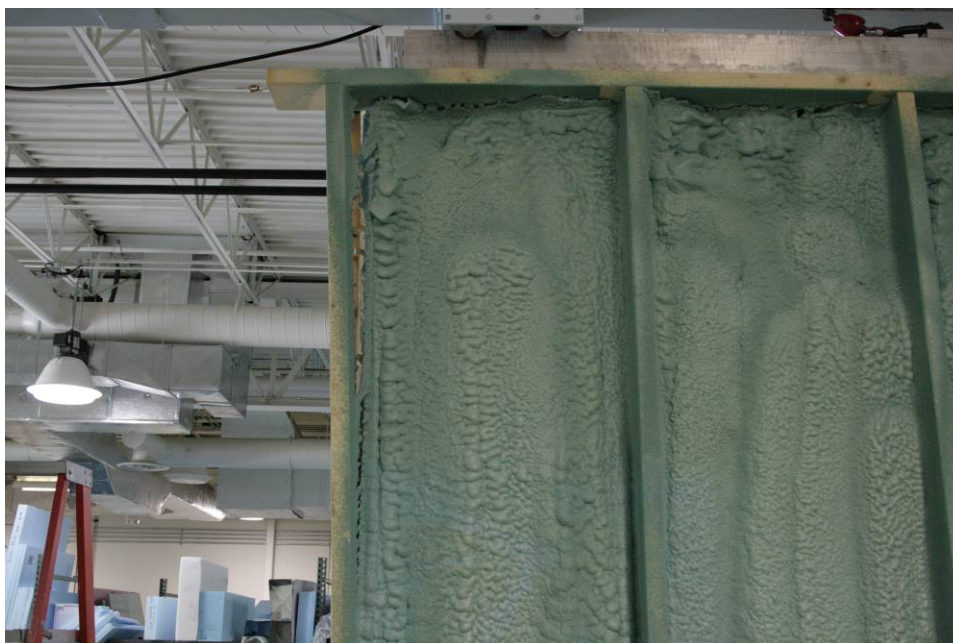
Figure 30. ccSPF tear propagation
