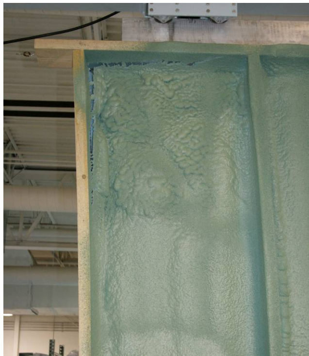
Figure 27. Stud flexure and ccSPF tearing
