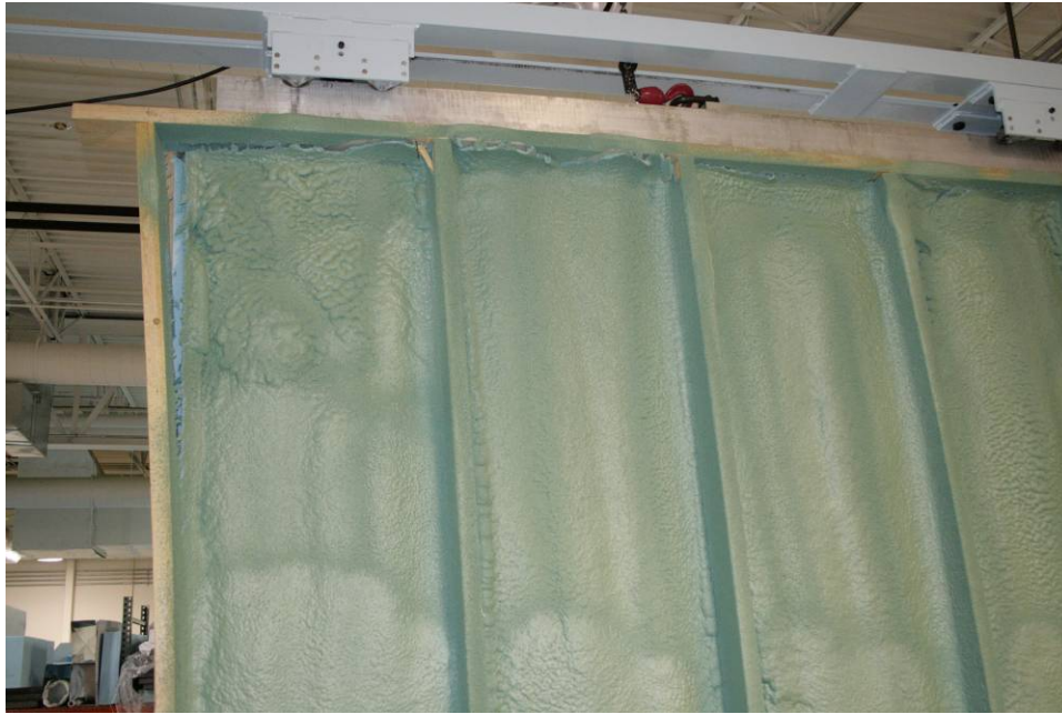
Figure 28. ccSPF tear propagation
