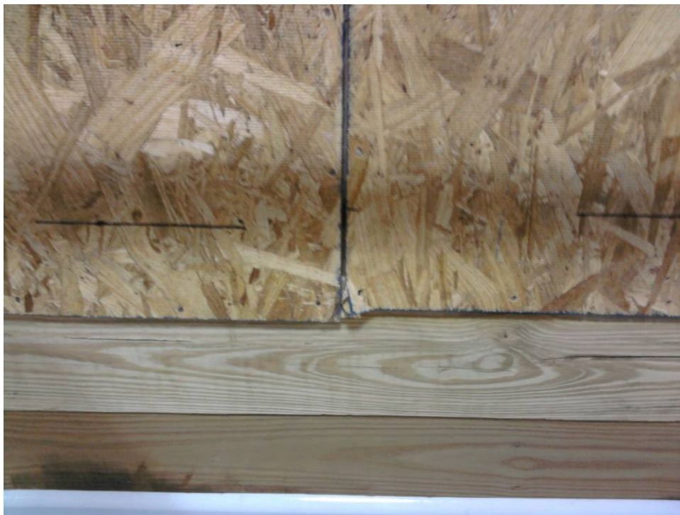
Figure 19. OSB failure at fastener
