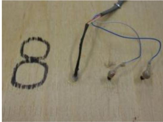
**Figure 6. Installed wood MC sensor and thermistor**
