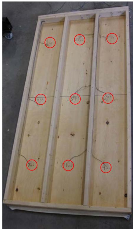
Figure 5. Location of wood MC sensors
