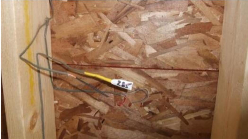
Figure 29. RH and temperature sensor installed in a stud bay (with MC pins installed below)
