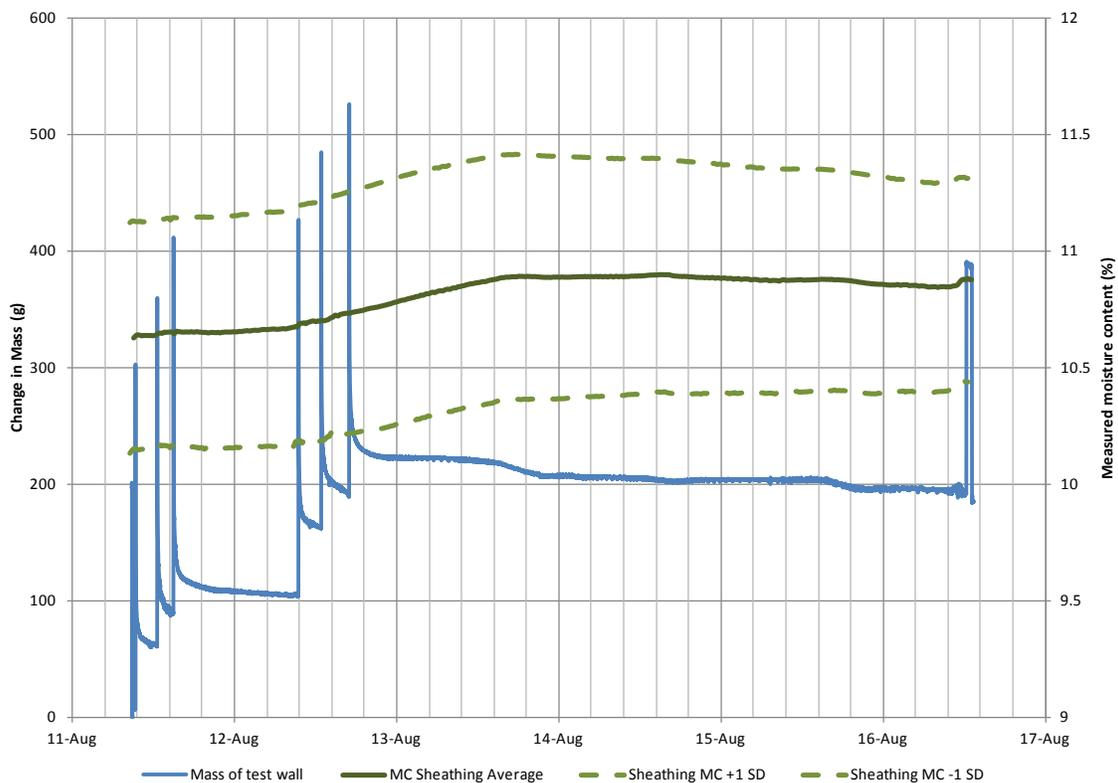
**Figure 13. Repeated drainage gap wetting analysis, smooth housewrap**
