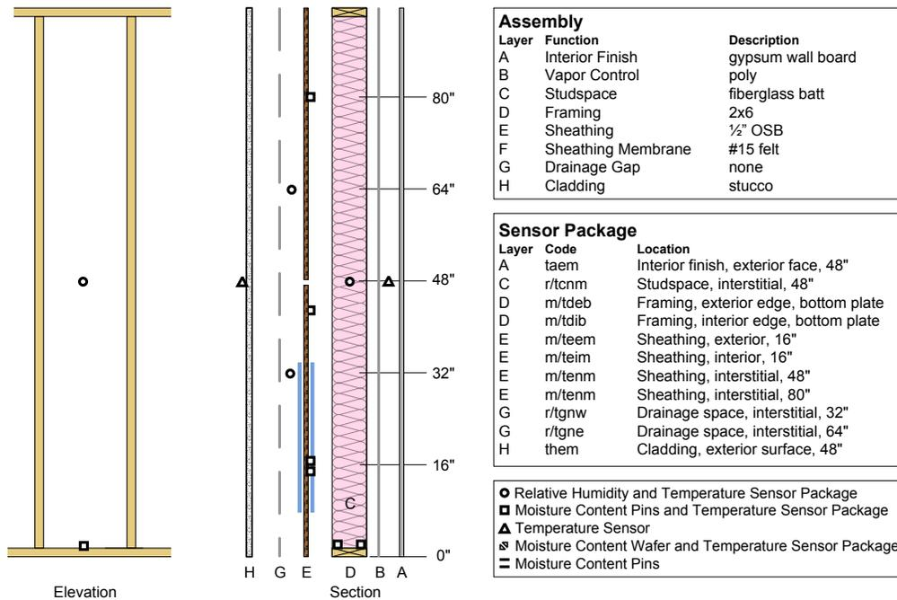
Figure 30. Typical wall construction and sensor configuration
