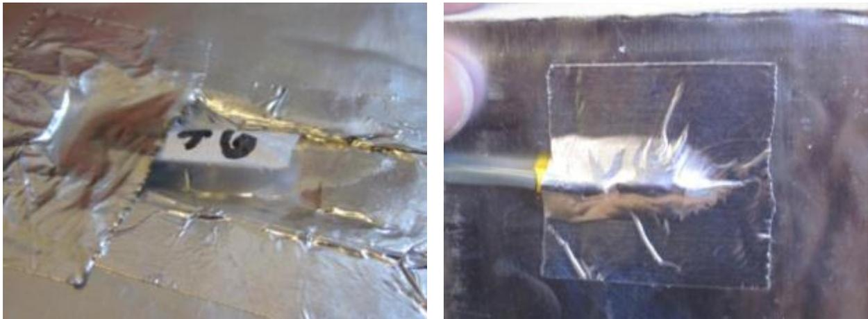
**Figure 15. RH sensor in the drainage space**
