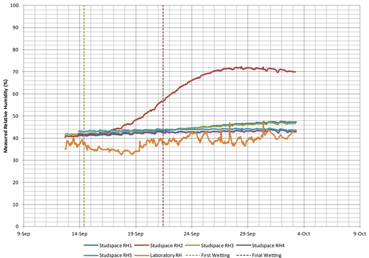
**Figure 22. Measured RH in the five stud spaces**
