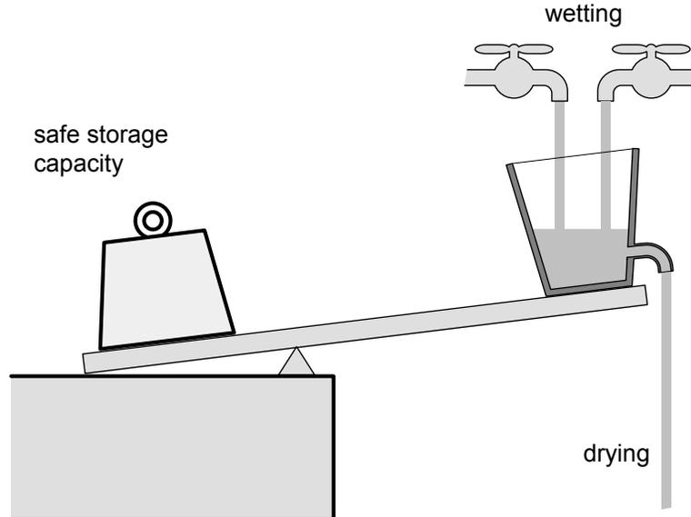
**Figure 2. Moisture balance of wetting and drying**
