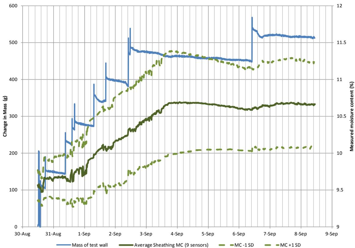
**Figure 14. Repeated drainage gap wetting analysis, corrugated housewrap**
