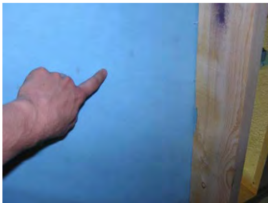
Figure 17: No penetration of Wall 1 at 30 fps
