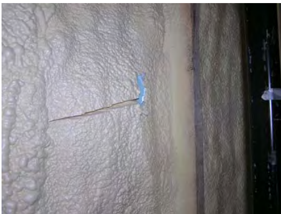
Figure 14: No penetration of Wall 2 and penetration of Wall 4 at 43 fps
