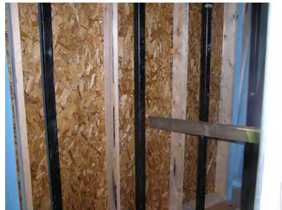
Figure 8: Stud penetration through all wall assemblies at 50 fps
