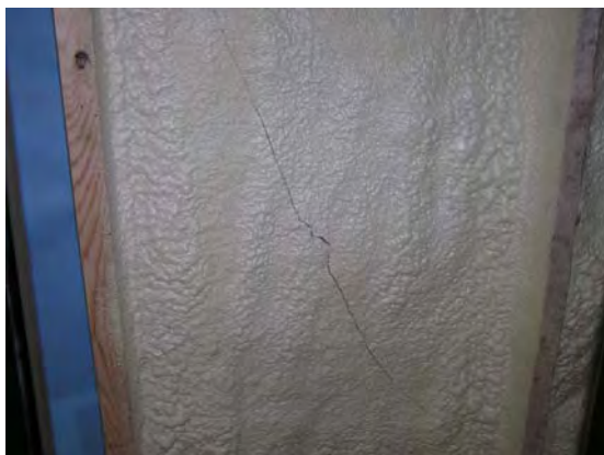
Figure 11: Cracking of both Closed Cell Foam and OSB Sheathing at 40 fps
