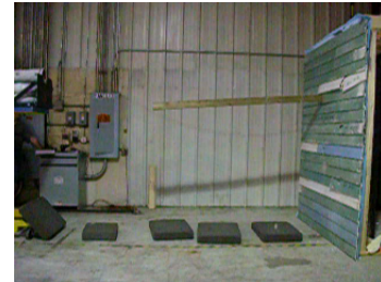
Stud penetrated cladding but not through Wall 2
