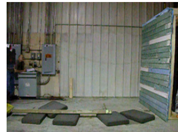
Stud on the ground after rebounding off of Wall 2
