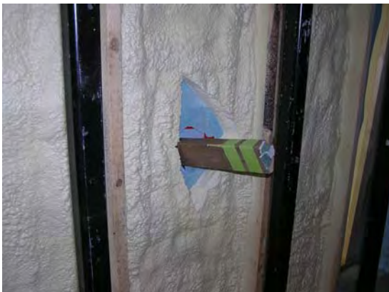
Figure 8: Stud penetration through all wall assemblies at 50 fps
