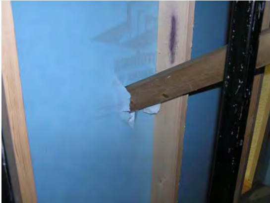
Figure 7: Wall 4 (Housewrap + ½ inch OSB Sheathing) fail at 50 fps
