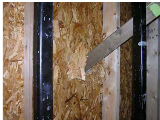
Figure 14: No penetration of Wall 2 and penetration of Wall 4 at 43 fps
