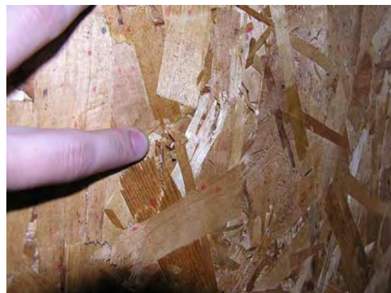
Figure 11: Cracking of both Closed Cell Foam and OSB Sheathing at 40 fps
