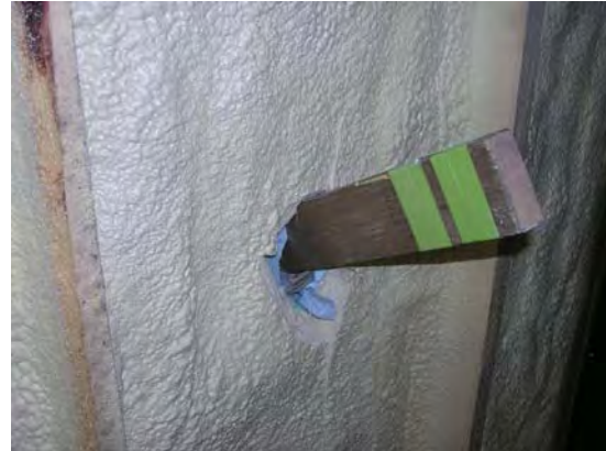
Figure 7: Wall 4 (Housewrap + ½ inch OSB Sheathing) fail at 50 fps
