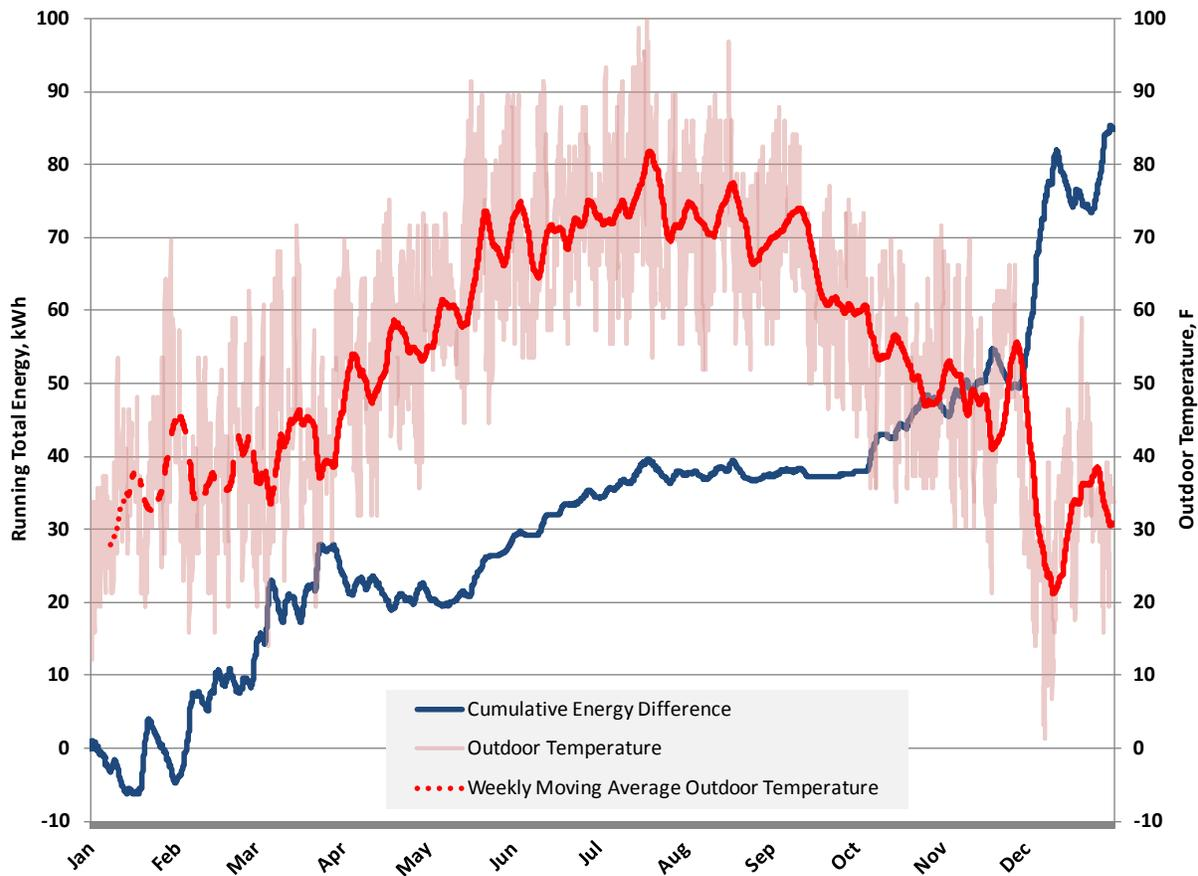
**Figure 12. Hourly HVAC energy for light frame and ICF wall systems**
