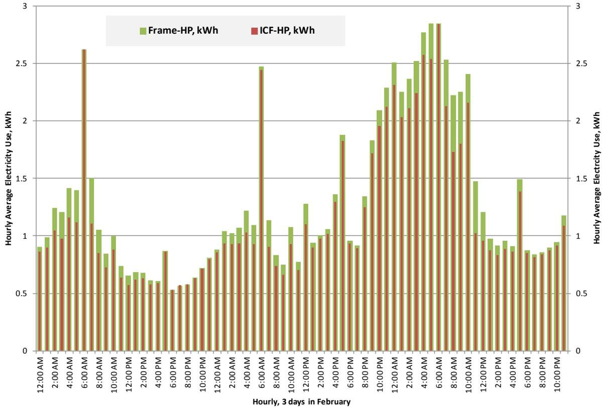
**Figure 11. Energy use comparison of ICF to light-frame wall system**
