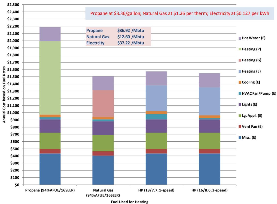
**Figure 9. Cost comparison for heating fuel sources**
