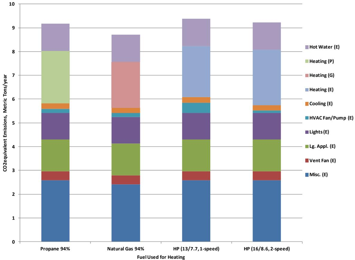
**Figure 10. Carbon factor estimates for different heating fuel types**
