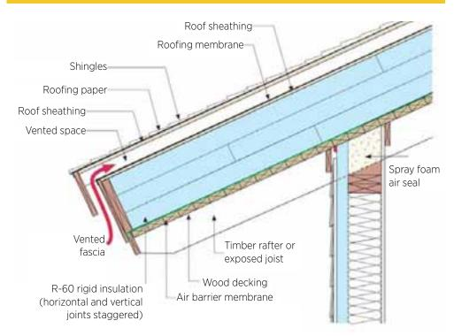
In regions with snow loads greater than 50  $lb/ft^2$ , the snow can provide enough thermal resistance to allow the roof cladding to be above freezing even when the air temperature is below freezing (one foot of snow = R-10 to R-15). To prevent ice damming with an unvented attic in these conditions, construct a "vented over-roof" over the top of the "unvented compact roof" (Source: Lstiburek 2011).
