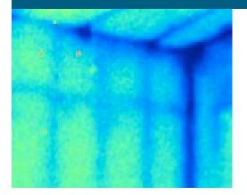
**Heat flow**. An infrared camera shows thermal bridging—heat moving through the wood framing into the home by conduction (Photo Source: DOE).
