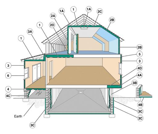
**Figure 2.1.** Building America research has identified key areas where insulation can improve a home's comfort, durability, and energy efficiency. (Source: 2008b)
