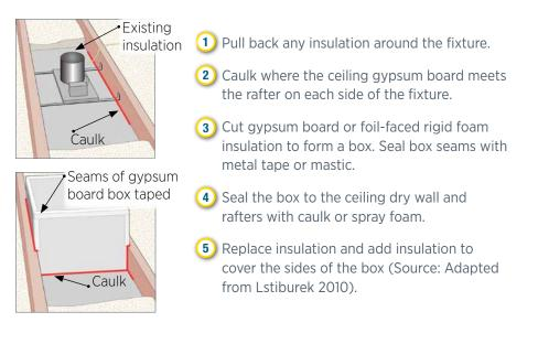
Holes in the top of the recessed can encourage the stack effect, pulling conditioned air up into the attic.
