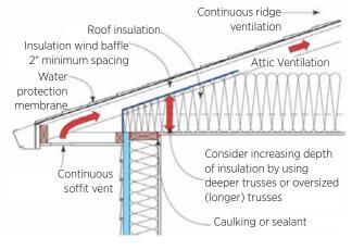
3 Vent the underside of the roof deck, with vent screens at every rafter bay and a 2-inch airspace under the sheathing where ground snow loads are greater than 30 lb/ft<sup>2</sup> (Source: Lstiburek 2011).
