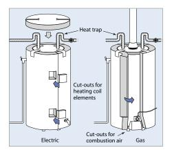
Electric and gas water heaters require different approaches to insulation. Gas and oil-fired water heaters are more difficult to insulate than electric water heaters. Their installation may be best handled by a qualified plumbing or heating contractor.
