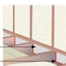
floor cavity openings • Seal edges with a continuous bead of caulk •—
