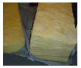
Unfaced fiberglass batt insulation
