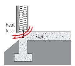
**Figure 5.20. Slab perimeter insulation**. Use rigid fiberglass insulation or boratetreated rigid foam approved for below-grade use (Source: DOE).
