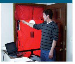
As part of the home performance energy checkup, your certified contractor will use a blower door test to measure wholehouse air leakage and determine places where insulation and air sealing are inadequate (Photo Source: PNNL).
