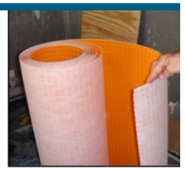
**Moisture control.** A dimpled plastic membrane can be placed over the existing concrete and under the the XPS to keep your concrete floor from wicking ground water into your home (Photo source: BSC).
