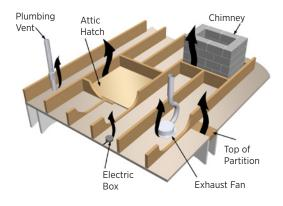
Figure 5.2. Ceiling holes. Homes are typically constructed with lots of holes in the ceiling for lights, pipes, vents, ducts, and chimneys. If the builder fails to air seal around these, air escaping through the gaps can carry moisture, possibly leading to mold and wood rot. These gaps must be air sealed before insulation is added to the attic (Figure Source: PNNL).
