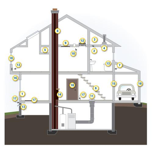
**Figure 5.1. Where to air seal.** Building America research has identified 19 key areas where air sealing can improve a home's energy efficiency, comfort, and durability. A certified home performance contractor can perform a home energy checkup to identify areas in your home that need air sealing (Figure Source: PNNL).
