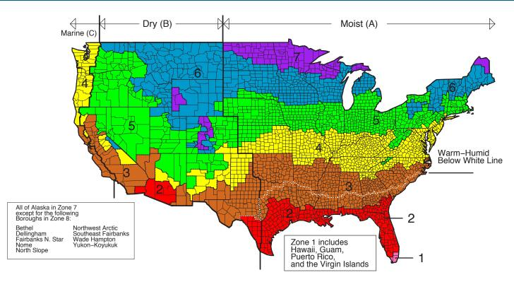
**Figure 2.2. IECC Climate Regions.** Designated by the International Energy Conservation Code (IECC) (Figure Source: 2009 IECC; Briggs et al. 2003).
