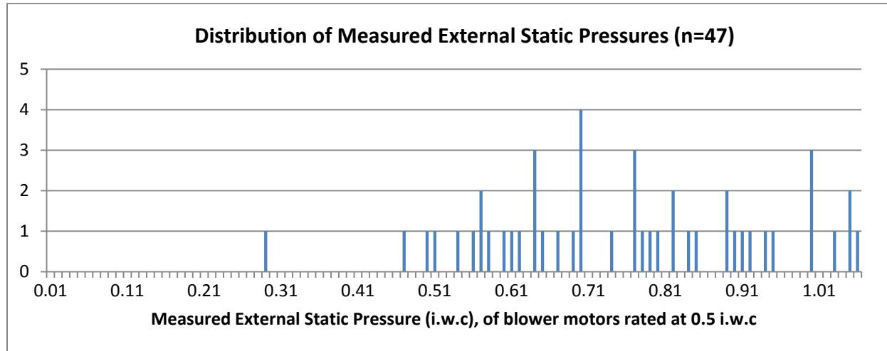
Figure 4. Measured ESP (i.w.c.) of blower motors rated at 0.5 i.w.c.
