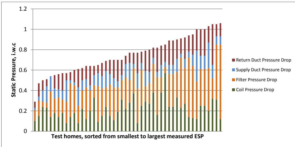
**Figure 5. Recorded static pressure drop, by component**
