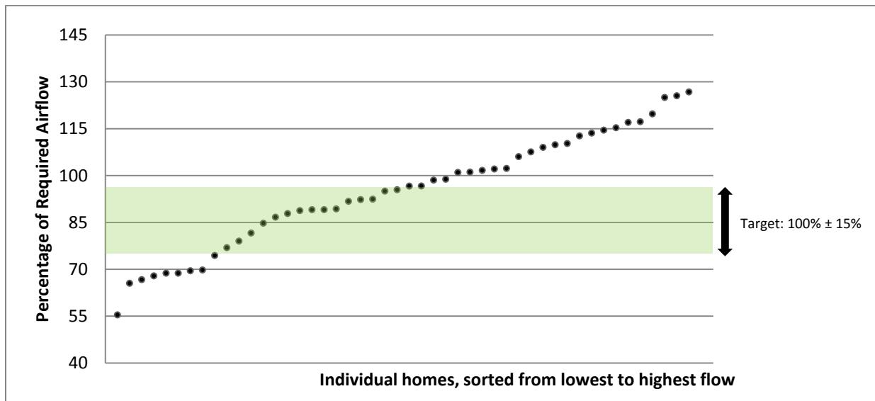
**Figure 19. Percentage of required airflow across heat exchanger as measured in the home**
