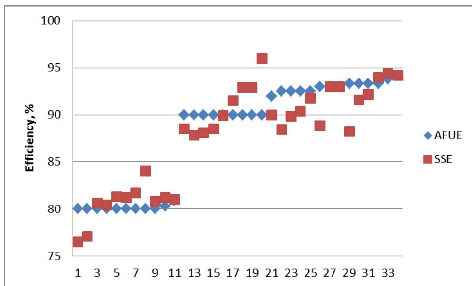
Figure 8. Label AFUE versus test-in steady state efficiency
