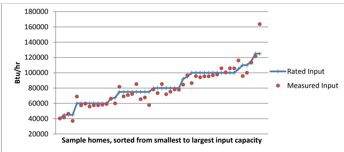
**Figure 6. Btu/h input to furnace**
