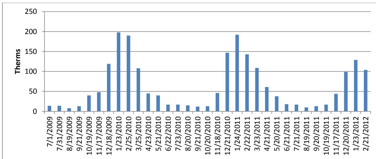
**Figure 10. Test home #1, natural gas usage pre- and post-retrofit**
