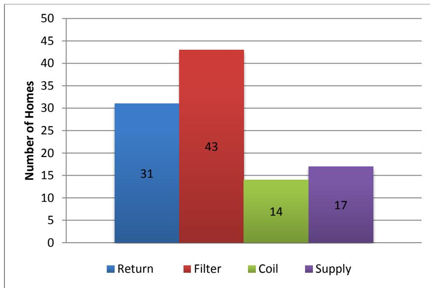
**Figure 21. ESP restriction, by location**
